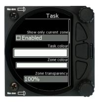
With this dialogue you can change the colour of the task line and turn point zone and modify the zone transparency and Zone line width.
