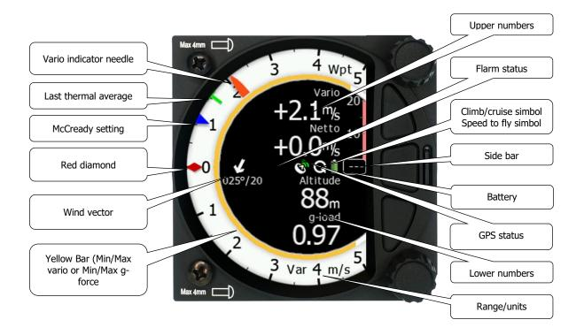
The Vario **Needle** can display: the Vario, Netto, Relative or Speed to fly value (Setup->Hardware->Indicator). The scale can be chosen in the range of +/-5 +/-10 or +/-20. Cursor style can be thin, medium or thick style. It can be linear or non-linear (setup->graphics->indicator). Within the software the range can be set to m/s, kts, km/h, mph or fpm (in Setup, Units, Vertical speed)
