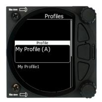
With the lower rotary knob, a pilot can scroll between different profiles, the profiles are stored within the internal storage of the S vario. Please note, the profiles are not stored on the SD card.
