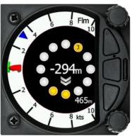
The central number and chevrons indicate if the Flarm target is below or above and by how many meters/feet. The number in the bottom right indicates the range in meters/feet. The numbers are related only to the closest or the most dangerous target.
