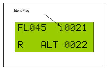
Pressing the ident key invokes the ident mode for 18 sec. Ident activity is shown by a in the middle of the upper line on the LCD screen, which starts blinking after 4 sec. as long as ident is acitve.
