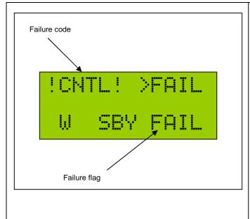
In case of failure, the system shows a union on the LCD screen. Additionally, a frequently repeated audible signal occurs. Both can be terminated by pressing the on/off key shortly.
