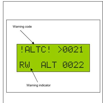
In case of warning, the system shows a on the LCD screen. Additionally, a frequently repeated audible signal occurs. Both can be terminated by pressing the on/off key shortly.
